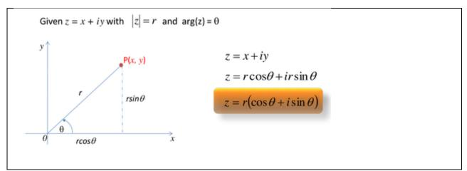
In this diagram, the complex number is denoted by the point P. The length OP is known as magnitude or modulus of the number, while the angle at which OP is inclined from the positive real axis is said to be the argument of the point P.
